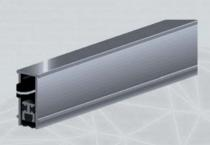
Consists of an extruded aluminium incorporating with a double vinyl seal which not only guarantees a perfect barrier, but also reduces unwanted noise level. The sealing distance may be altered by turning the adjusting screw above the activating roller at the end of the fitting.
