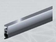
A general purpose seal for doors and windows and is especially designed for timber casement windows and all hinged doors. The PTS profile is manufactured from rigid uPVC incorporating a soft vinyl insert which acts as a seal against the closing frame.
